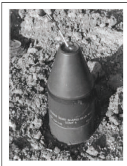
Figure 2-51. Priming Shaped Charges With an MDI
