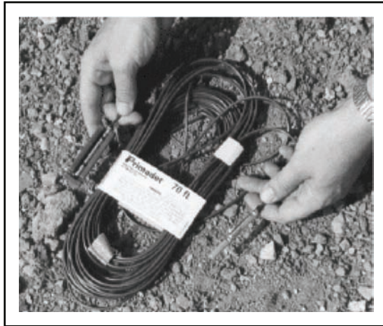
Figure 2-43. M15 Delay Blasting Cap
