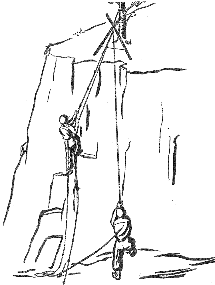
Figure 41. Vertical hauling line.
