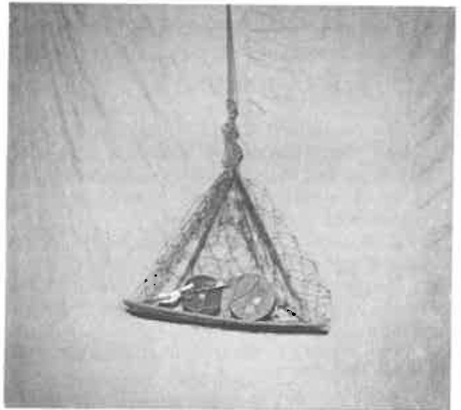
Figure 21. Containers for 8-inch atomic projectile, M422, configuration II (assembled storage configuration), in cargo net prepared for external transport. Note use of nylon cord around the net.
