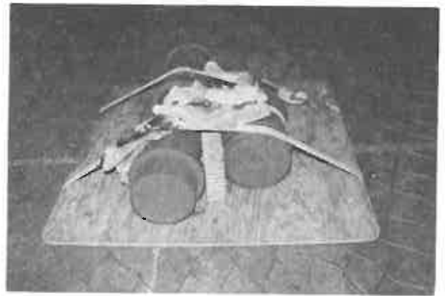
Figure 20. Containers for 8-inch atomic projectile, M422, configuration II (assembled storage configuration), secured to plywood. Note that running ends of straps are folded and taped.
