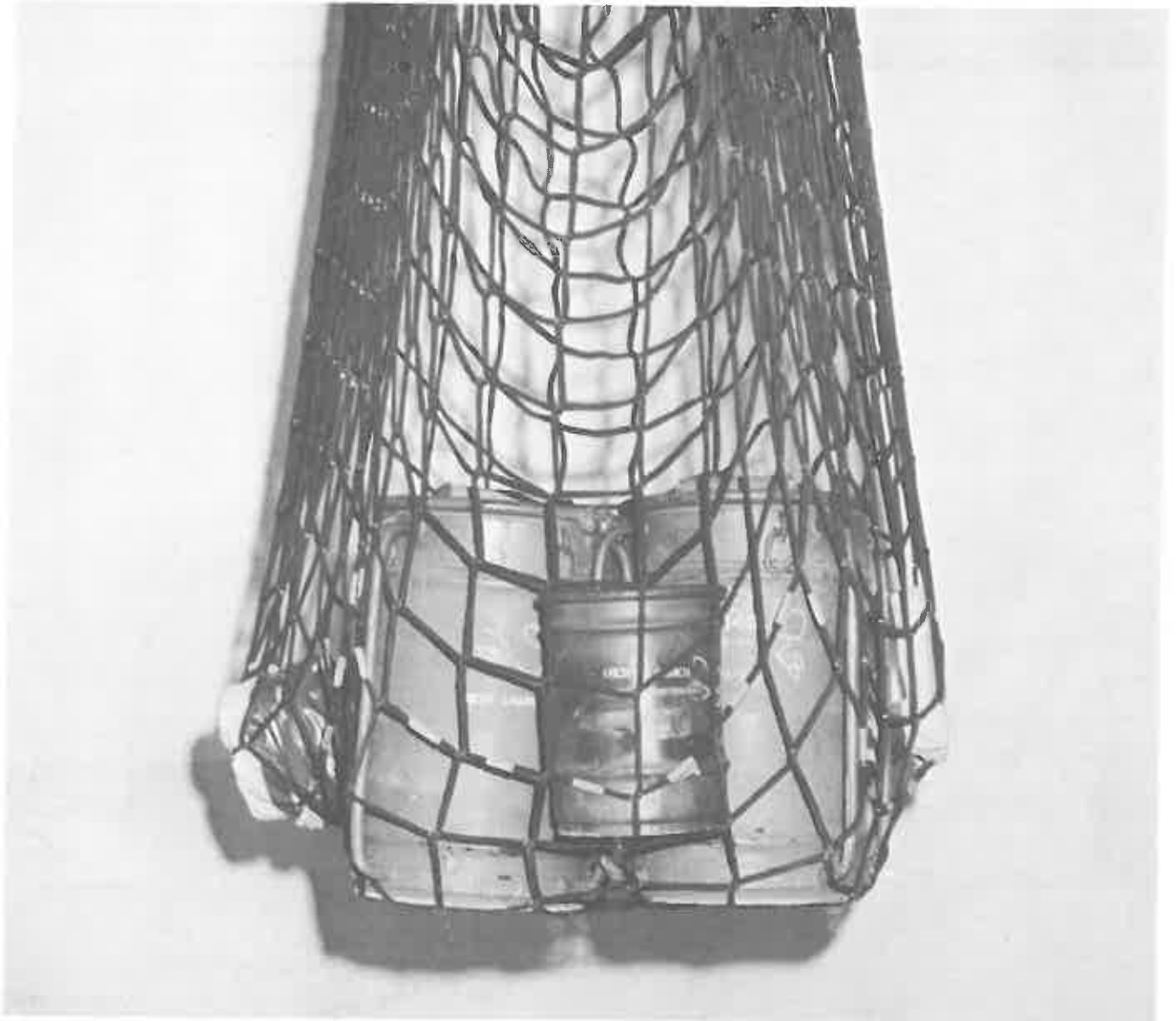
Figure 5-3. Test lift of containers for one 8-inch atomic projectile, M422, in 5,000-pound-capacity nylon cargo net.
