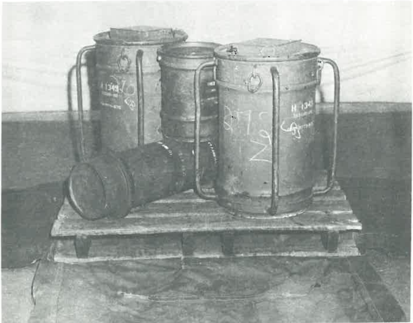
Figure 5-5. Containers for one one 8-inch atomic projectile, M422, palletized in center of cargo bag.
