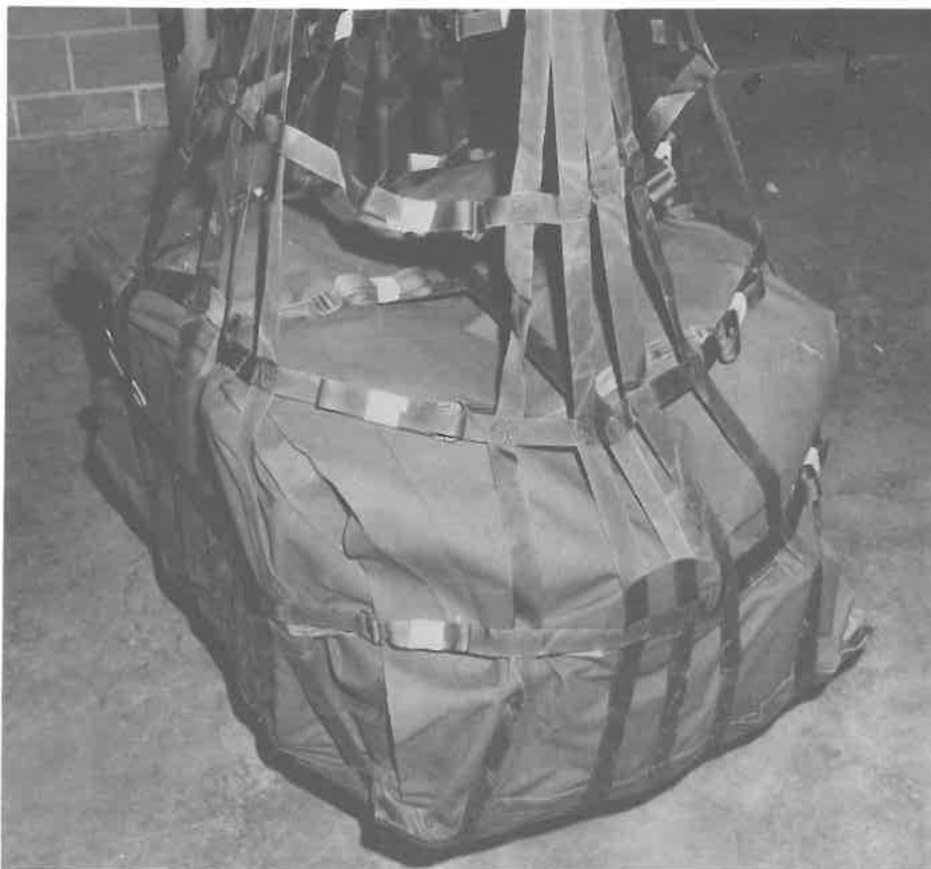
Figure 5-9. Lower and upper lateral straps fastened around the load and secured at corners of cover.
