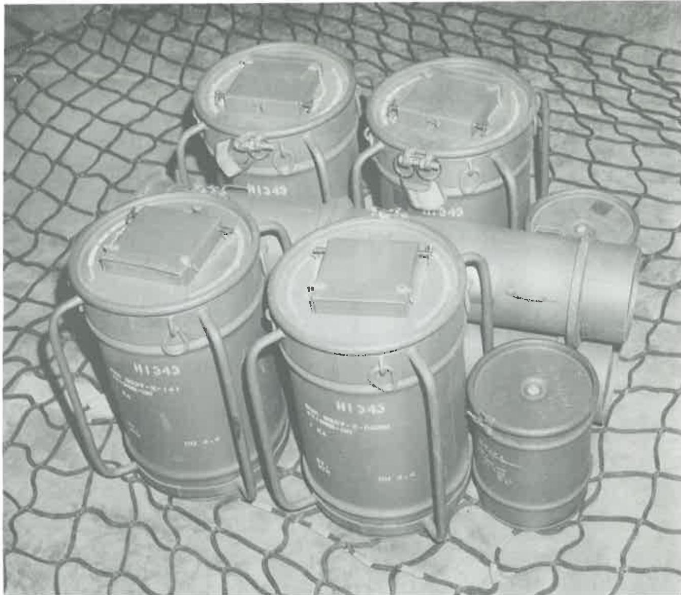
Figure 5-2. Containers for two 8-inch atomic projectiles, M422, in 5,000-pound-capacity nylon cargo net. Padding not yet applied to projectile cases, M500.
