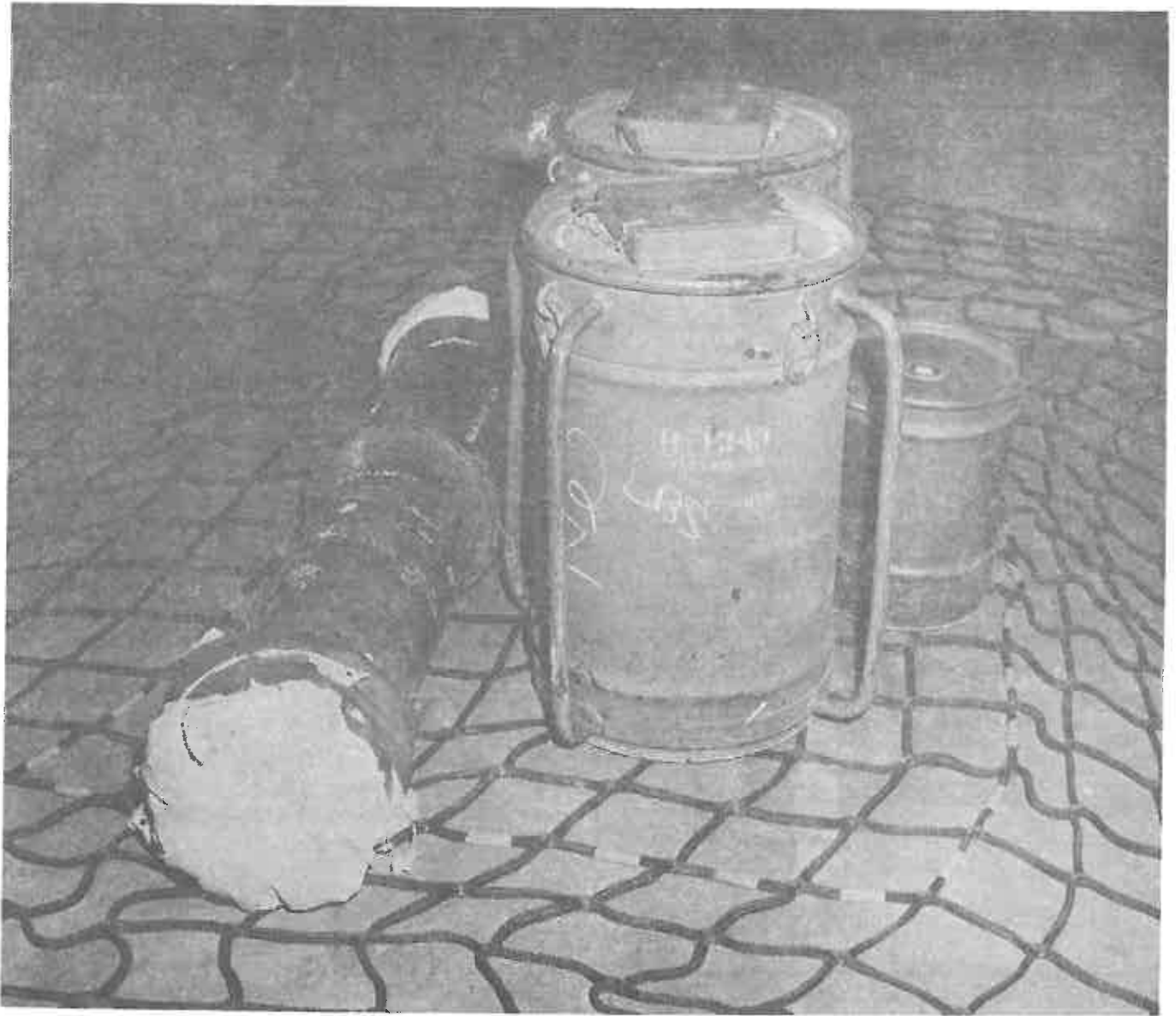
Figure 5-1. Containers for one 8-inch atomic projectile, M422, in 5,000-pound-capacity nylon cargo net. Note padding on projectile case, M500.
