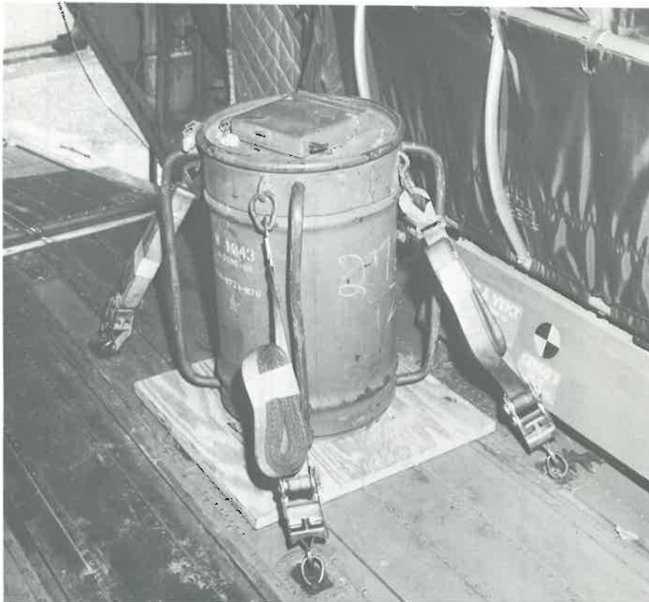
Figure 4-14. H1343 container positioned on shoring and tied down in CH-47 helicopter. The second H1343 container is out of view on right side of helicopter.
