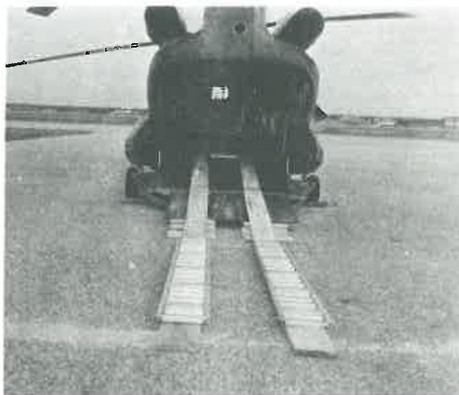
Figure 4-1. Rolling, blocking, and parking shoring and conveyors positioned for loading Nike-Hercules warhead section shipping and storage container, M409, into CH-47 helicopter.
