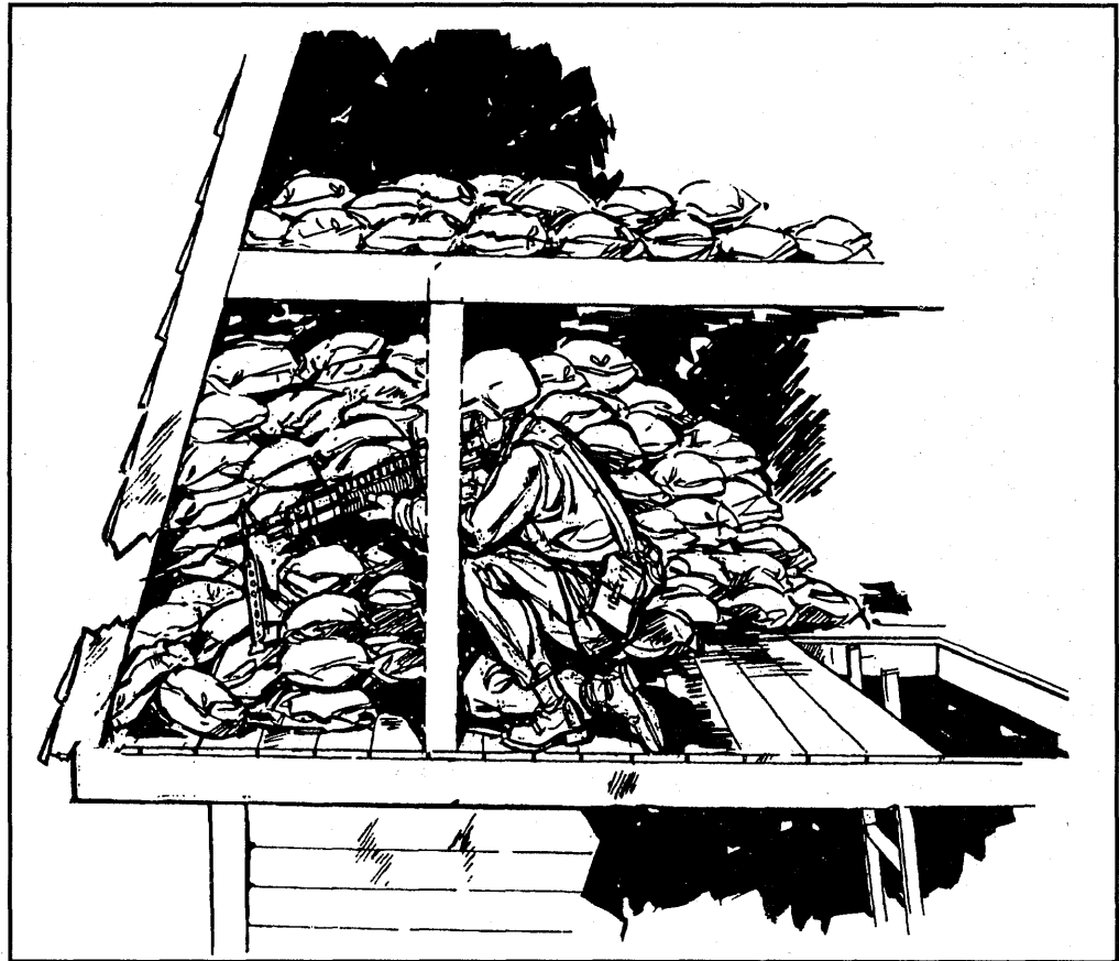
Figure 5-41. Firing platform built under roof.
